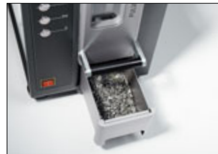
Comminution of ferrous alloys with the Jaw Crusher PULVERISETTE 1 premium line – 6.5 mm gap width
