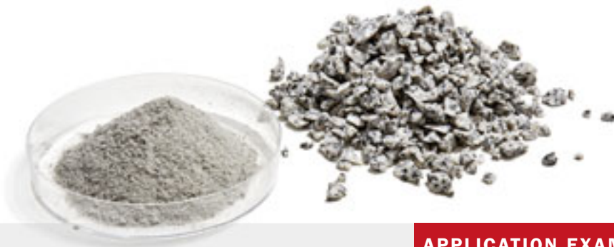
Optimal preparation of a granite sample using the Planetary Micro Mill PULVERISETTE 7 premium line
