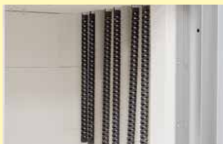
Vertically mounted SiC rods and optional perforated air inlet tubes of the debinding system in a high-temperature furnace
