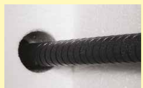
Furnace chamber with high-quality fiber materials and SiC heating rods on both sides of the furnace
