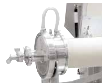
Water-cooled vacuum flange (gas supply system 2)
