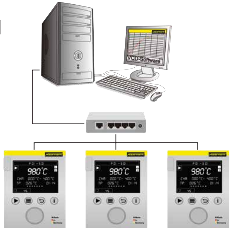
Example lay-out with 3 furnaces
