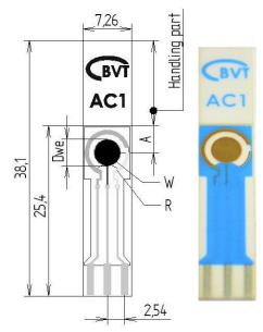
without contamination of active area. The handling part can be broken off and sensor can be inserted in the standard BVT flow cells.
