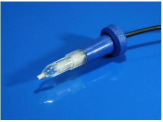
electrode (CEc) is designed for measurements with thermostated cell TC4, TC5, TC6, TC9.
