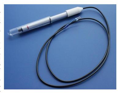
used measuring apparatus, with internal resistance of above 10<sup>9</sup> - 10<sup>12</sup>. Standard electrical connecting cable is 0.8 to 1 m. coaxial cable with BNC connector. The work with ion selective electrodes is time effective, requires an only small amount of chemicals, and a friendly price of measuring equipment MPH471.
