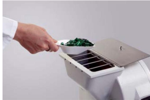
The quality of every product or material analysis depends on the quality of the sample preparation. It is therefore extremely important to consider all the individual milling parameters in order to make an informed choice: material properties of the sample such as density, degree of hardness, feed size, sample quantity, grinding time and desired final fineness, any abrasion of the grinding parts, temperature sensitivity or residual moisture – all these factors are significant.
