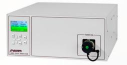
If a standard one or two channel UV/Vis detector is not adequate for preparative purifications, a diode array detector offers simultaneous multi-wavelength or full UV/Vis spectrum - peak purity - analysis for complex chromatographic purifications.
