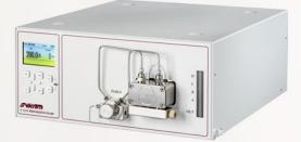
The S 1535 Preparative Pump, with a flow rate range of up to 250 ml/ min and pressure range up to 400 bar with stainless steel pump heads and optional built-in low pressure mixing quaternary gradient mixer
