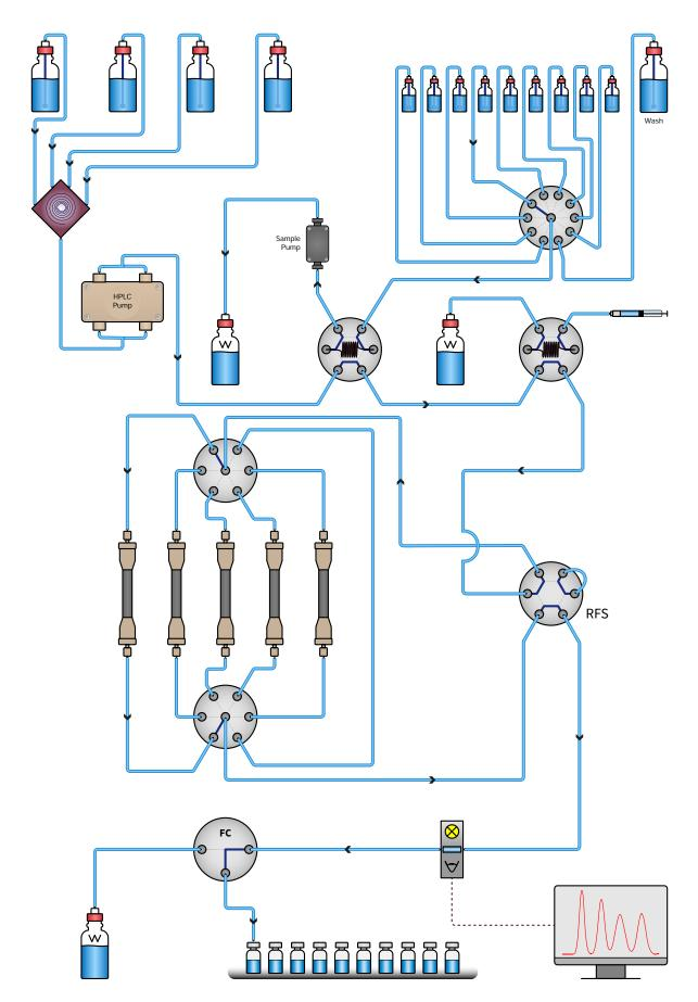
A low pressure quaternary gradient system with manual and automatic injection. Column switching up to 6 columns, or 5 columns and one bypass for flushing or sanitizing routines. Reversed flow switching (RFS) for counter-current elution or column regeneration. Fraction collector.
