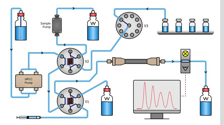
Shown above: the S 5400 sampling flow path. Valve 1 is the manual injection valve. Valve 2 is the automatic injection valve. Valve 1, valve 2 and the sample pump are integral parts of the S 5400 sampling module. Valve 3 is the optional external valve for automatic sampling of up to 10 samples.
