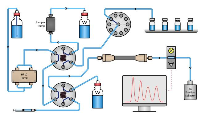
An isocratic configuration with manual injection port and automatic sample injection of up to 10 samples (fraction collector omitted)
