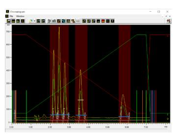
Visualisation of signals: fraction collection windows, gradient profile A/B, collection threshold, fraction number
