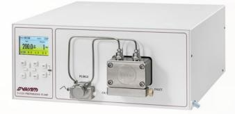
The S 1525 Preparative LC pump is the largest heavy duty pump of the preparative LC product range. The S 1525 pump is available with four flow rate ranges. These are 150, 250, 500 or 1000 ml per minute. Each available as stainless steel version or as metal-free PEEK versions.
