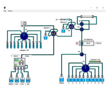
Monitoring and dynamic control of the system. Example shown: a quaternary gradient system with manual and automatic sample injection, reversed flow switching and fraction collection
