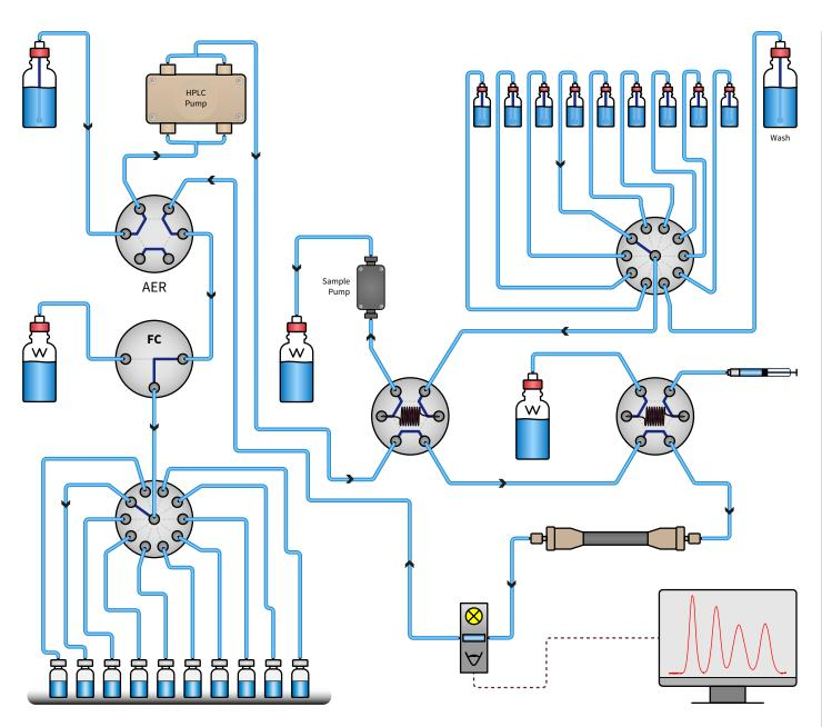
An **isocratic system** with automatic eluent recycling (AER) possibility and manual and automatic sample injection. Fraction collection with a 10 port valve enabling large volume collection, useful for stacked (repeating) sample injection routines.
