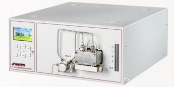
The S 1535 Preparative LC Pump is available as a 150 ml/min and a 250 ml/min version and a pressure range of 400 bar with stainless steel pump heads, and up to 350 bar with PEEK pump heads.
