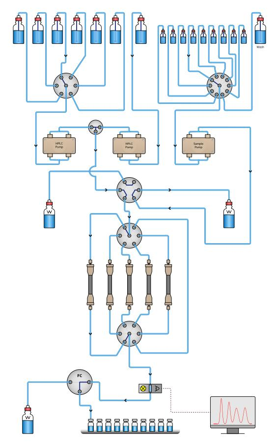
A **binary high pressure gradient system** with additional 6-channel buffer/eluent selection for the primary pump. A sampling pump for large volume sample injection and a sampling valve for connecting up to 10 sample containers. Column switching up to 6 columns, or 5 columns and one bypass for flushing or sanitizing routines. Fraction collector.
