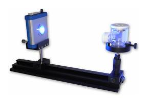
Optionally included with the Optical platform is a water jacketed 40ml glass cell that fits the cell positioning clamp. The glass cell is equipped with a quartz glass window to allow the light to pass through. A lid with a sealing ring is provided with 3 openings for the counter electrode, reference electrode and working electrode.
