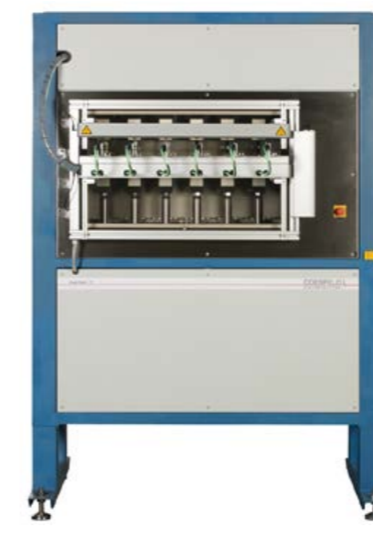
Fig 5: Coesfeld 6 Station Creep Test System
