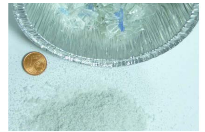
Fig 2: PET bottles comminuted with 1 mm sieve
