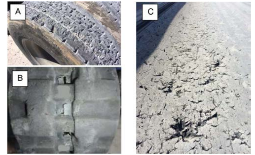
Fig 1. The Cut & Chip wear phenomena of a truck tire tread (A), a rubber track (B) and a conveyor belt (C).
